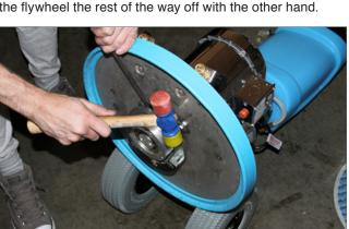
**5.** Use the 15/16" wrench to hold the jam nut in place and use a mallet to strike the flywheel counterweight to tighten the flywheel against the jam nut.
