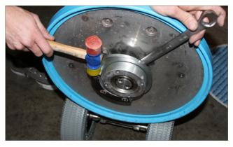
2. Hold the jam nut, located between the flywheel and motor, in place with a 15/16" open-end wrench. Using a mallet, tap the flywheel counter-clockwise to loosen.
