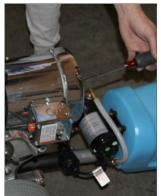
**3.** Remove the plastic plug from the top of the motor and hold the motor shaft in place by inserting a flathead screwdriver into the top of the shaft on top of the motor. Loosen the flywheel the rest of the way off with the other hand.
