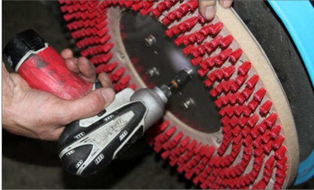
1. Remove the pad driver assembly by removing the four bolts with a 7/16" wrench or socket.
