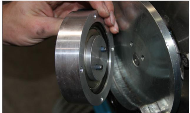
4. Insert the Allen bolts into the new bearing and line up the bolts with the holes on the flywheel.
