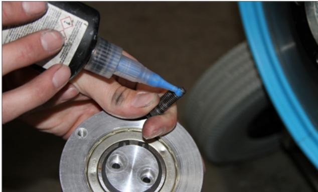
3. Remove the Allen bolts from the bearing and apply Blue Loctite®.
