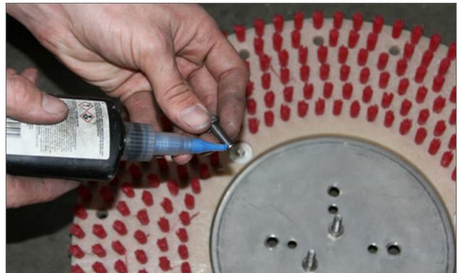
6. Apply Blue Loctite® to the pad driver bolts and bolt it back onto the machine.
