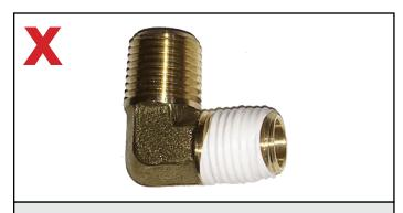
**DO NOT** use Teflon sealing tape or hand tools to install the fittings that screw directly into the pump head. The excesive stress to the threaded pump ports will lead to immediate head cracking.
