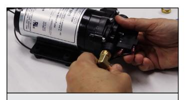
Hand tighten the fitting. Then, use a wrench to gently position the fitting after hand tightening. No more than a ¼ turn past snug should be employed. **DO NOT** overtighten the fitting. Overtightening will lead to cracking.
